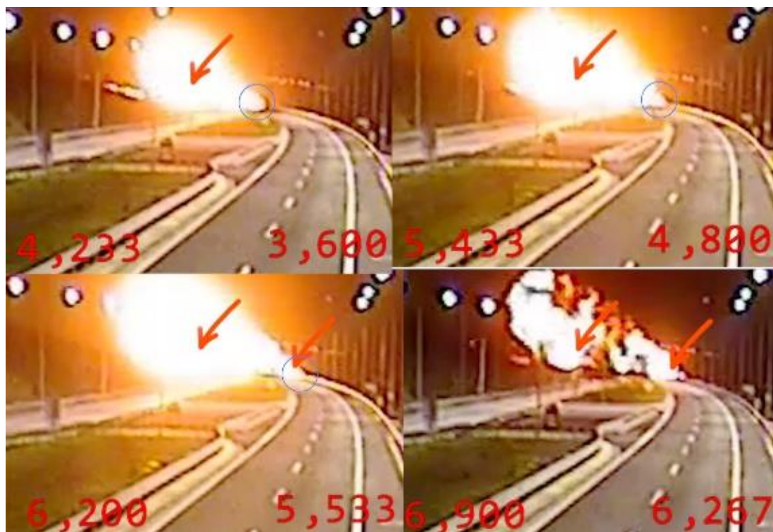
Figure 29. Second stage, fireball (left side of pictures) and fire plume (right side of the pictures)
