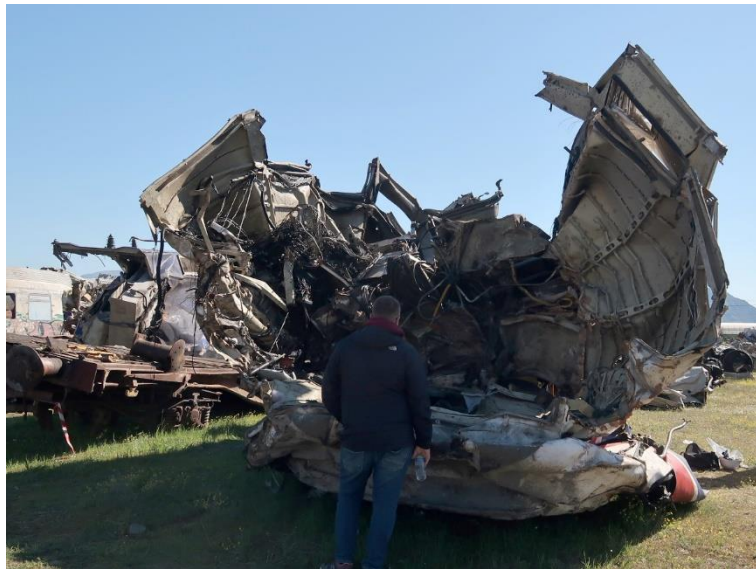
Figure 16. Front view of the locomotive 120-022, roof missing.
